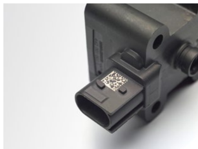
Code marking on difficult placements
