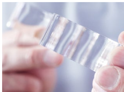
Flame-polished result. Cut up to 40mm acrylic.
